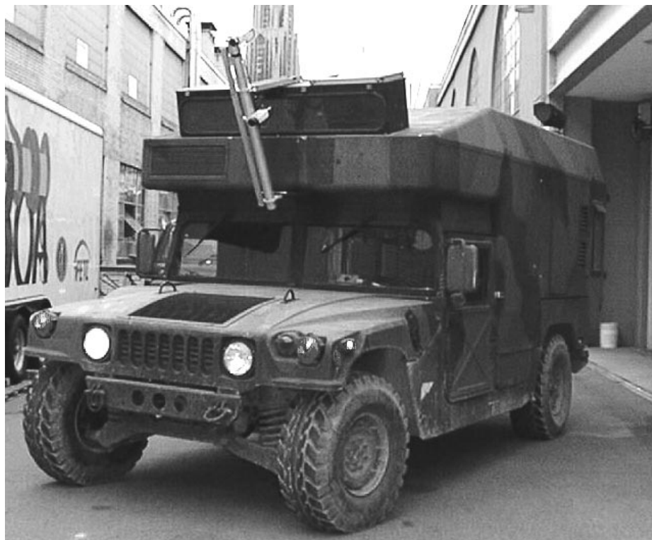
Figure 1 Side view of the CMU HMMWV vehicle used for the TUGV project with stereo cameras mounted above the cab.
