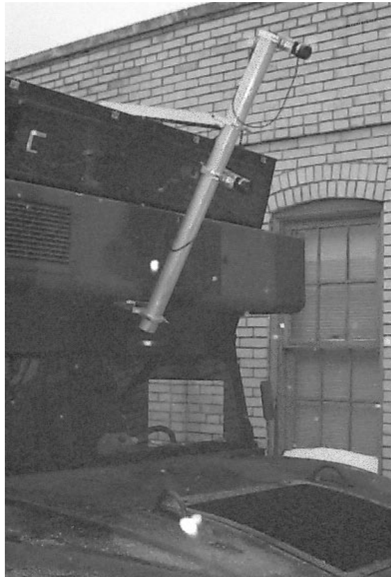
Figure 3 Vertical baseline stereo camera mounts. The baseline between the cameras can be extended to up to 1 m. The mast is tilted downwards at 30 degrees.
