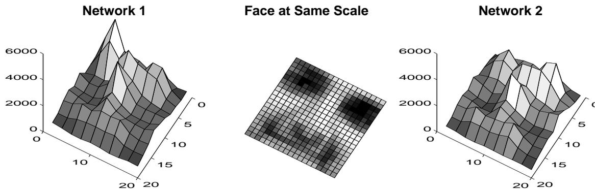
**Figure 5:** Error rates (vertical axis) on a small test resulting from adding noise to various portions of the input image (horizontal plane), for two networks. Network 1 has two copies of the hidden units shown in Figure 1 (a total of 58 hidden units and 2905 connections), while Network 2 has three copies (a total of 78 hidden units and 4357 connections).
