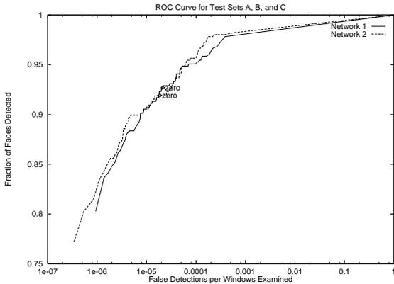
**Figure 6:** The detection rate plotted against false positives as the detection threshold is varied from -1 to 1, for two networks. The performance was measured over all images from Test Sets A, B, and C. Network 1 uses two sets of the hidden units illustrated in Figure 1, while Network 2 uses three sets. The points labelled “zero” are the zero threshold points which are used for all other experiments.
