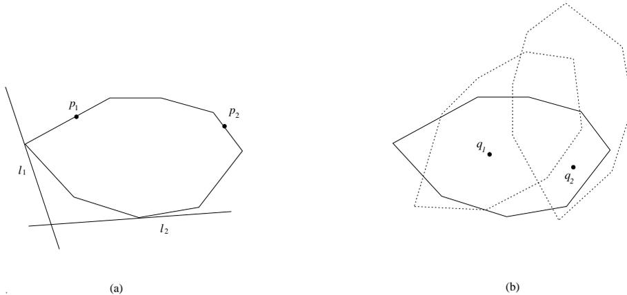
**Figure 1:** Geometric sensing of an 8-gon. (a) The case of a continuum of possible poses: Four incidence constraints  $p_1, p_2, l_1$  and  $l_2$  suffice to determine the pose. (b) The case of a finite number (three) of possible poses: Only the containment of two points  $q_1$  and  $q_2$  must be checked to determine the real pose.
