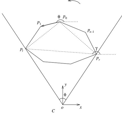
**Figure 4:** A convex polygon  $P$  rotating in a cone. The pose of  $P$  is denoted by the position of vertex  $p_0$  and the angle  $\theta$  between directed edge  $\overrightarrow{p_0 p_1}$  and the  $x$  axis. The space of orientations  $[0, 2\pi)$  is partitioned into closed intervals, each defining an elliptic curve that describes the corresponding locus of  $p_0$ .
