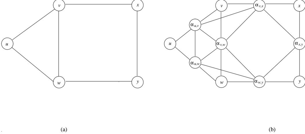
**Figure 10:** An example of reduction from Independent Set to 3-IS. (a) An instance of Independent Set. (b) The constructed 3-IS instance:  $\alpha$  vertices are added to increase the distances between the original vertices by exactly one.
