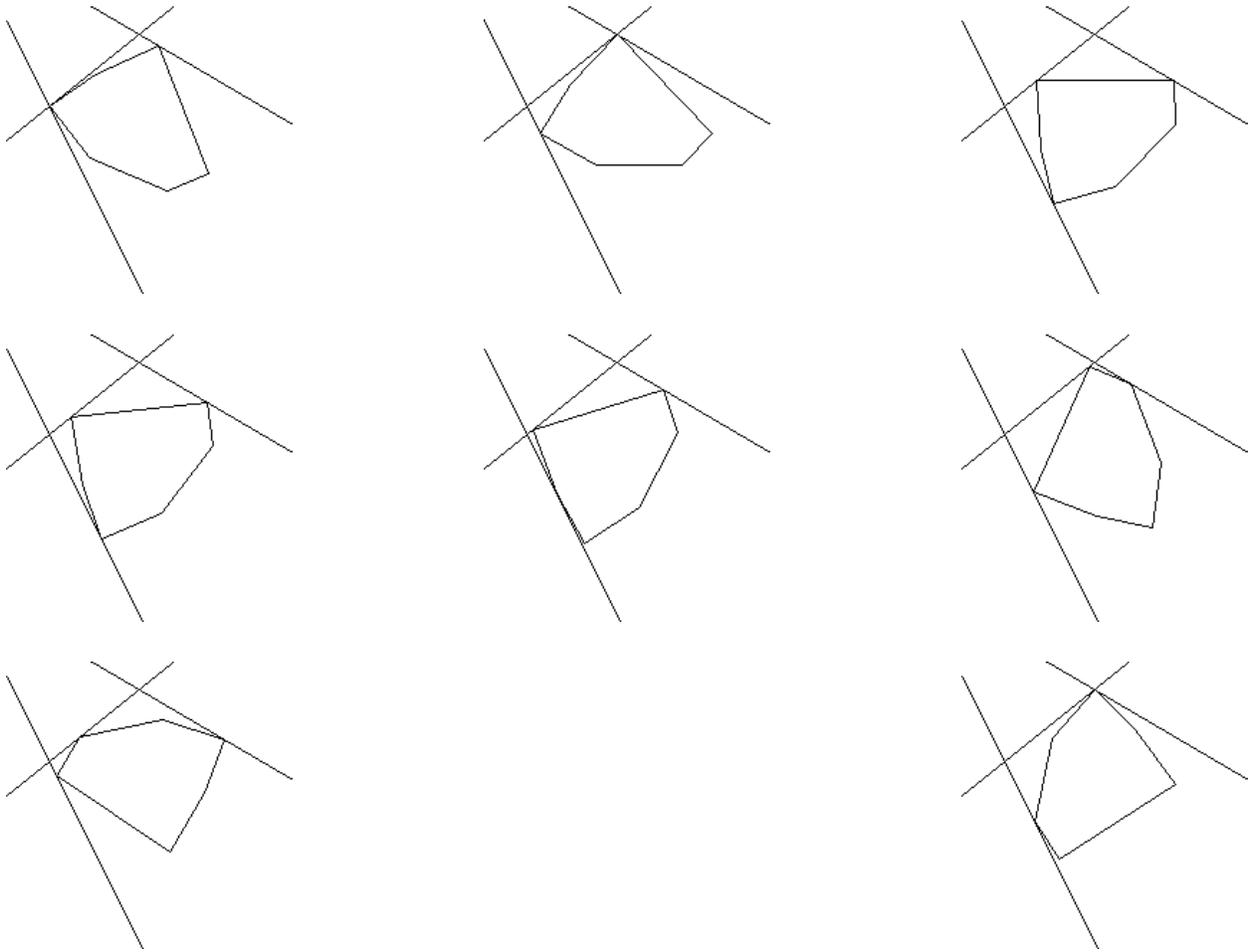
**Figure 5:** Eight possible poses for a convex 6-gon bounded by three supporting lines (as taken from a sample run). The first one represents the real pose whose supporting lines as shown were generated randomly; the remaining seven represent all other poses consistent with the supporting line constraints. Notice in this example that three of the eight poses occurred when a vertex of the polygon coincided with an intersection of two supporting lines.
