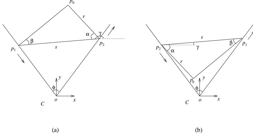
**Figure 3:** A triangle sliding in a cone. Vertices  $p_1$  and  $p_2$  move along the two sides of cone  $C$ . The locus of  $p_0$  is an elliptic curve (possibly degenerating into a line segment) parameterized by the angle  $\gamma$  between directed edge  $\overrightarrow{p_2p_1}$  and the  $x$  axis. There are two different cases: (a)  $p_0$  is above edge  $p_1p_2$ ; (b)  $p_0$  is below edge  $p_1p_2$ .
