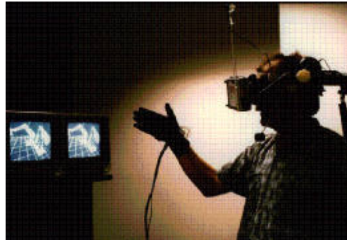
Figure 12 An operator in the VIEWS system controlling a Puma 560 manipulator arm. The operator’s view is visible in the monitors to the left.
