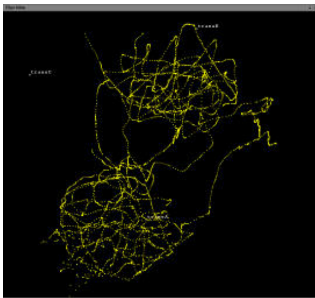
Figure 7 A screen image of the Map View window, showing telemetry tracks of a vehicle during an exploration mission.
