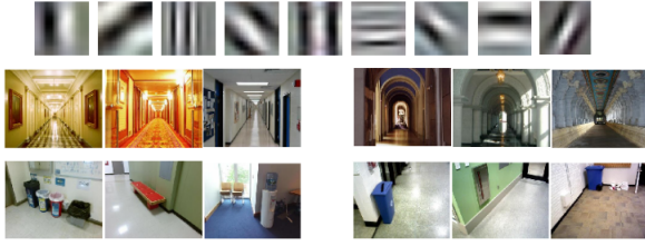
Fig. 8. CNN visualization. Top row: selected filters from first layer. Bottom two rows: top three activation images of selected four neurons in layer pool5. Each set represents certain corridor configurations such as straight forward corridors and left turning corridors.
