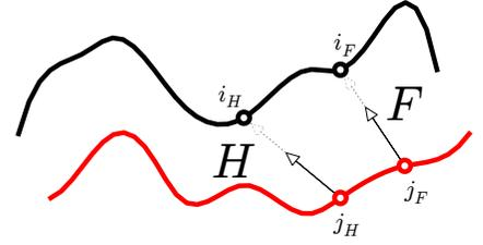
Fig. 4: The negative analytical gradient of the Fréchet and Hausdorff distance steps to decrease the distance.
