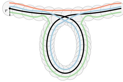
Fig. 3: The one way (orange) and two way (green) Hausdorff distances are constrained to be in the safe zone while the Fréchet distance (blue) forces us to pass through the safe zone in order.
