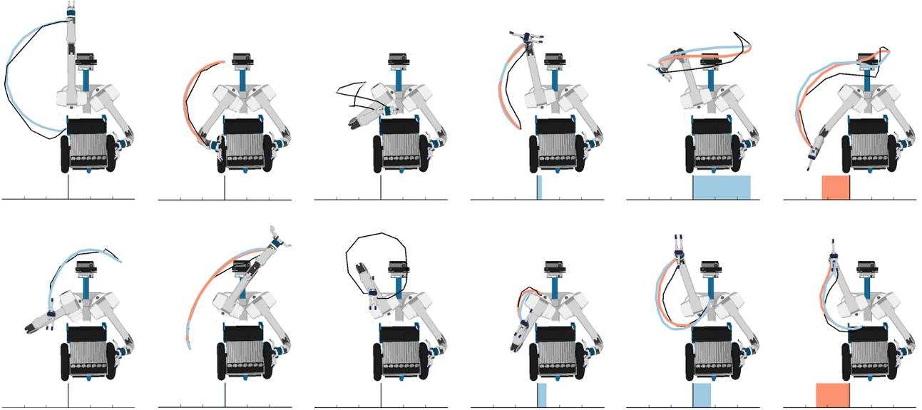
Fig. 5: The demonstration is shown in black. The path optimized according to the Hausdorff and Fréchet metrics are in orange and blue, respectively. The bars below show the difference between the Fréchet error of the two optimized paths.
