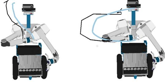
Fig. 10: The original reference path is given in black and the blue path is translated 10 cm.
