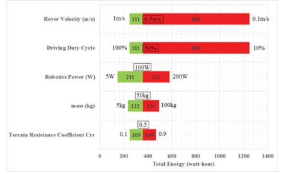
Fig. 2: Influence of Different Rover Parameters on Total Required Battery Energy to Accomplish a 2km Traverse
