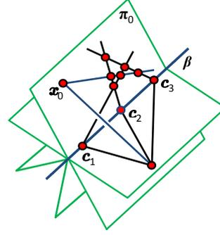
Figure 5. For collinear pinholes, there exists a single scene plane  $\pi_0$  in the pencil passing through the baseline  $\beta$  that contains  $x_0$  and for which the condition  $T_0 = 0$  is ambiguous.
