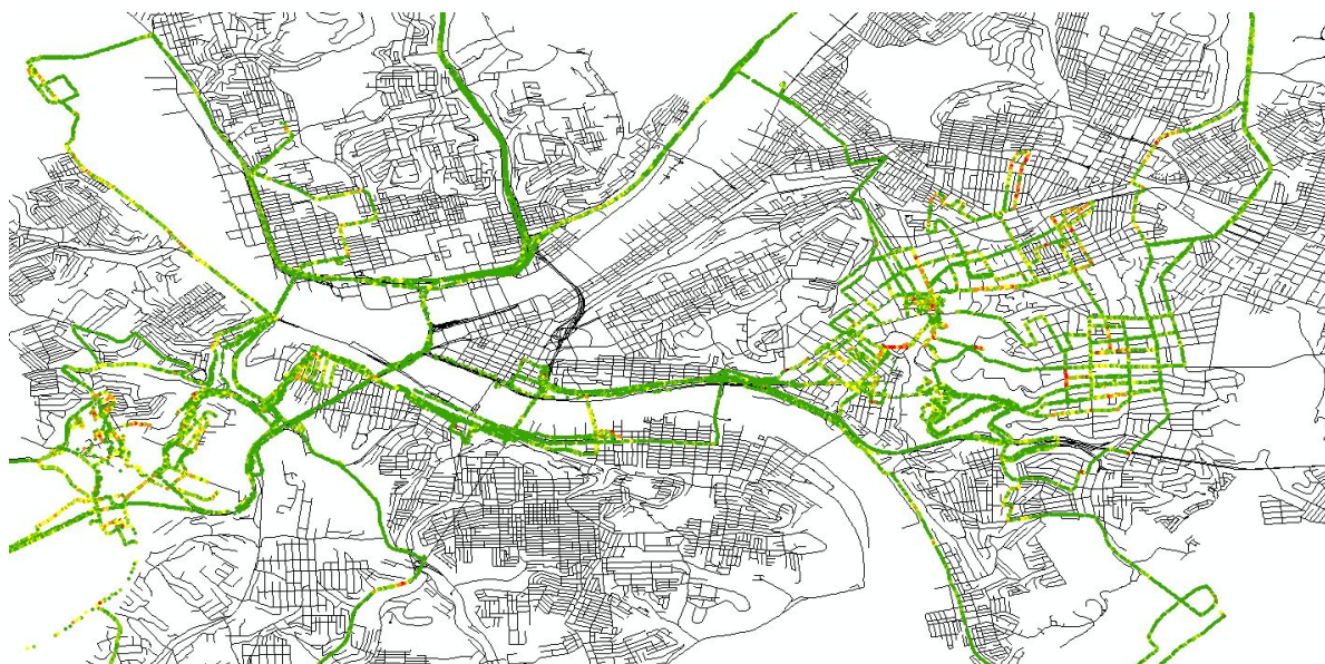
Figure 15: Citywide road damage severity due to cracks: green - low to none, yellow - medium, red - severe. Note that only a subset of the city's road network has been covered.
