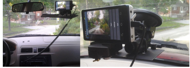
Figure 1: Mounting of the smart camera. On the left one can see its position within the windshield and the power cord from the cigarette lighter. On the right is a closeup of the suction cup, the shield, the snap-mount, and the display after startup.
