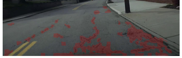
Figure 10: Classifier result: detected crack regions are shown in red.
