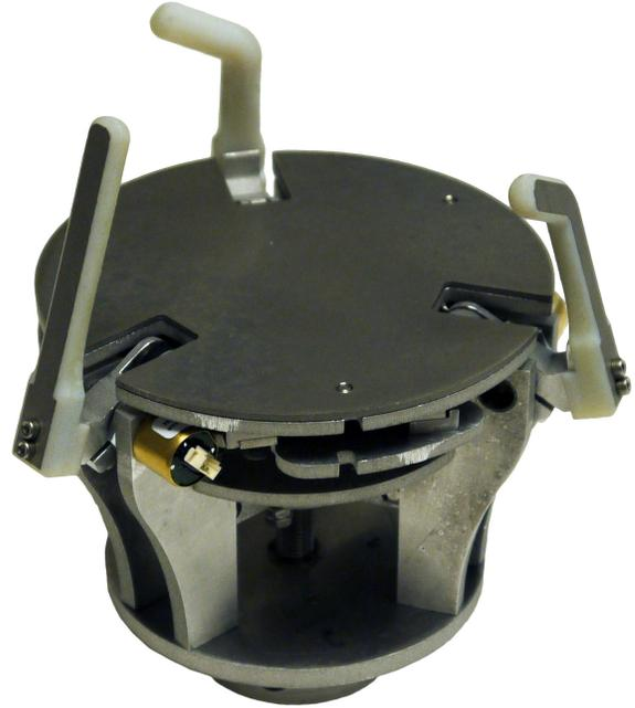
Fig. 1. Force Sensing Palm installed on the MLab P3 Simple Hand. The circular outer edge of the palm is 101.6 mm in diameter.
