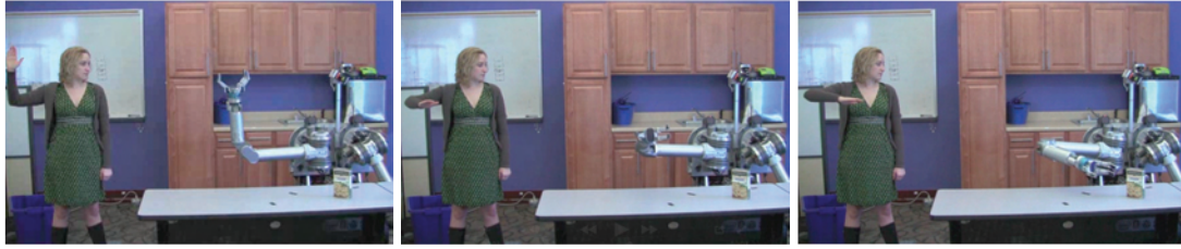
Fig. 11. A user with an unusual strategy for teleoperating. She moves the robot one joint at a time.
