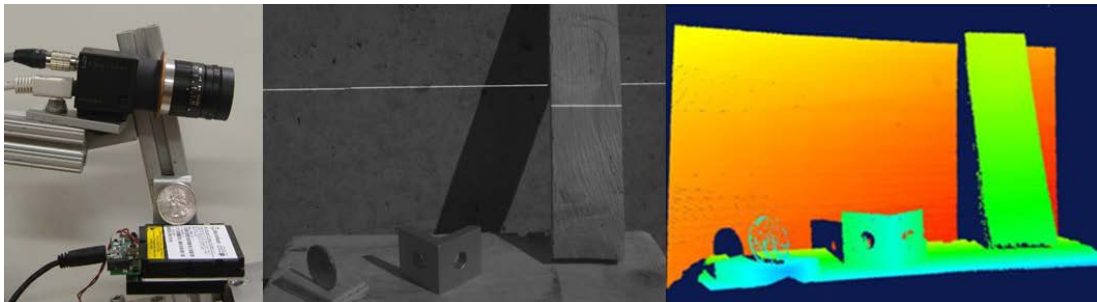
Figure 1 Left: Camera and PicoP® projector. Middle: Scene in direct sunlight with one laser line. The ambient sunlight is suppressed by the fast shutter and a bandpass filter. Right: Reconstructed 3D scene, color indicates depth
