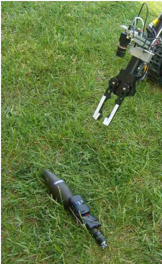
Figure 7 Scanning line striper mounted on a robot arm and observing a mockup IED.
