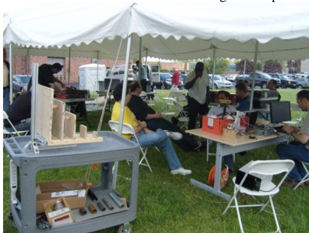
Figure 2 Measurement setup. The scanning line stripper was sitting on one table. The calibrated target was placed on a cart.
