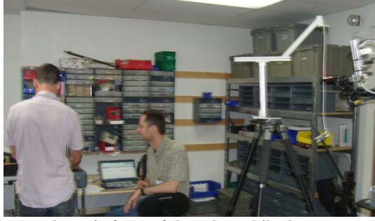
Figure 8 Setup for GUI testing: A wire was hung in front of the robot while the operator (left person) was guiding the arm and the gripper.
