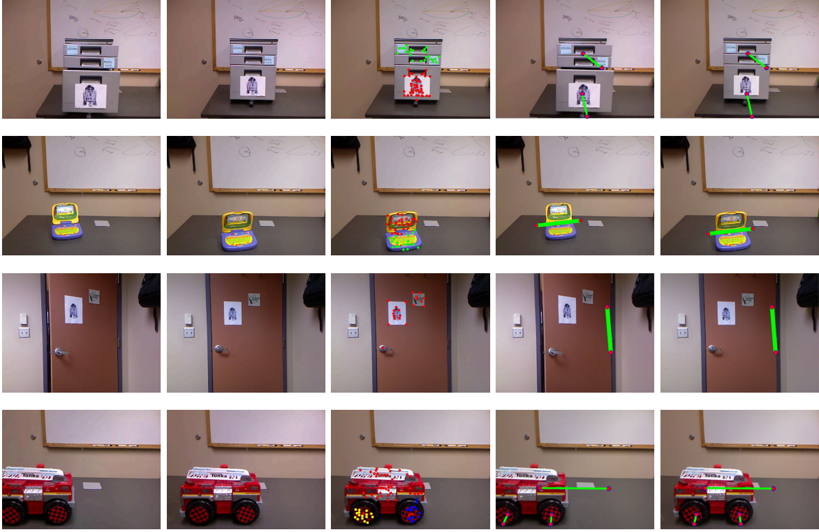
Fig. 6: Experimental results showing the process of segmenting a scene into its individual objects. Left to right: The first column shows the object before the interaction; the second column shows the object after the interaction; the third column shows the results of clustering the tracked features into rigid bodies; the fourth and fifth columns show the results of joint detection obtained for the first two rows.
