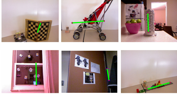
Fig. 7: Additional experimental results showing the detected joint for more everyday objects: a checkerboard (revolute), a door (revolute), a paper-towel (revolute), a stroller (prismatic), a toy train (prismatic), and a window (prismatic). The detected joints are marked in green.
