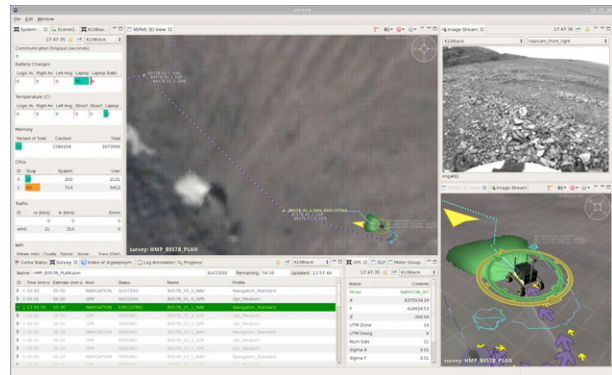
Fig. 7: The Visual Environment for Robotic Virtual Exploration (VERVE) is an interactive 3D user interface for monitoring robot operations.
