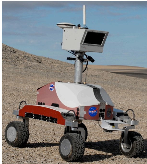
Fig. 5: The K10 planetary rover is a MER-class robotic rover testbed. K10 “Red”, is seen with an ILRIS-3D Lidar system at the top of its mast.
