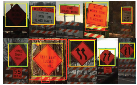
Fig. 2. Some sign detection output images are shown. The thick (yellow) rectangles outlining the signs represent the overlap between the ground truth rectangle (green) and the detection output (red). In the top row, from the left, the images represent examples of W20-1, R22-1, G20-2, W21-19, and R2-2-2 workzone signs. The bottom row includes examples of W1-4, W1-4L, W1-4R, W4-2R, and W4-2L. We include these identifiers of workzone signs for completeness and also later represent the sign target classes. Viewed best in color.
