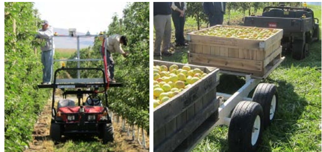
Fig. 1. Two vehicles in the Autonomous Prime Mover family. (Left) Orchard workers thinning green fruit from onboard an autonomous platform. (Right) Workers using the autonomous vehicle as a “bin dog” to increase harvest efficiency.
