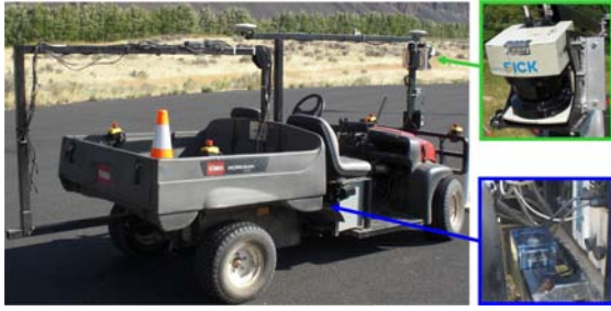
Fig. 2. Laurel Autonomous Prime Mover. In this work we use only the steering and wheel encoders, low-cost IMU (blue box on the bottom right) and one laser scanner (green box on top right) for obstacle detection.
