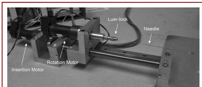
**FIGURE 2.** The needle-steering system developed for use in the cadaver trials.
