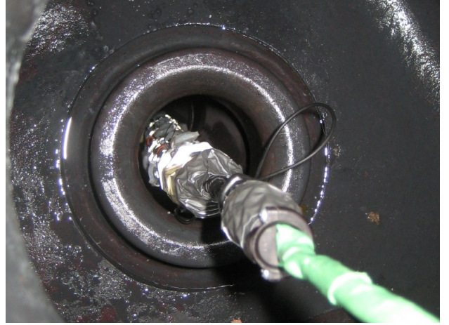
Fig. 1. View of a snake robot crawling inside of a turbine.
