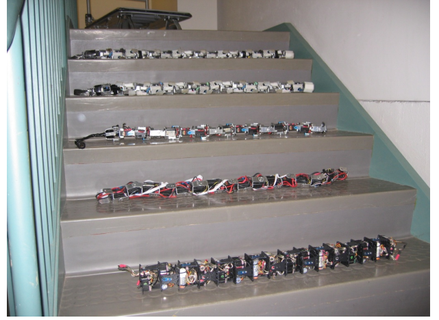
Fig. 2. Progression of modular snake robot development - older robots are at the bottom of the image.
