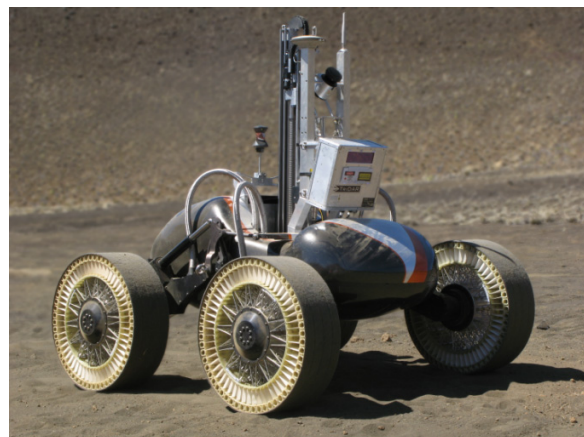
Figure 1. The Scarab rover has an actively controlled suspension that can change wheel base length.
