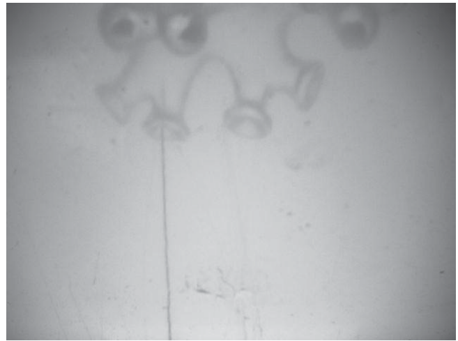
Figure 4. Final result from test in vitro in kidney tissue phantom. The needle tip is visible inside one of the calyces of the kidney at the top of the figure.
