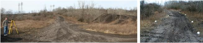
Fig. 13. Multiple close range scans were taken of the area using the Leica ScanStation2, then aligned using the spherical fiducials (right). The overlapping scans produced a dense, uniform pointcloud suitable for use as a groundtruth dataset.
