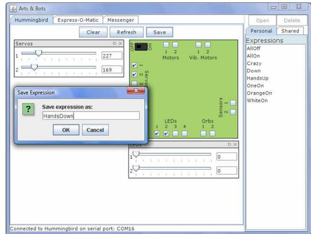
**Figure 1:** The programming software. Sliders are used to set the state of servos, LEDs, and other robot components. The set of state parameters are saved as an “expression” which can later be linked together with other expressions to form a simple sequential program.
