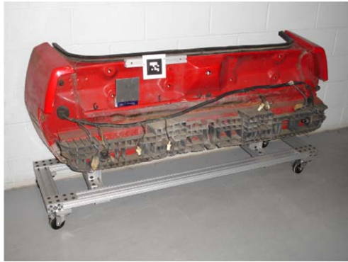
Fig. 2 Our task board is the back end of an actual vehicle. A fiducial is mounted near the target hole
