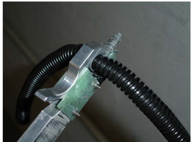
Fig. 4 A spring-loaded gripper holds a plug, ready for insertion into the target hole on the task board
