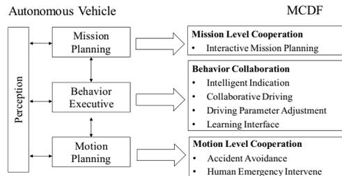
Fig. 2. Mission-Behavior-Motion Level MCDF Block Diagram
