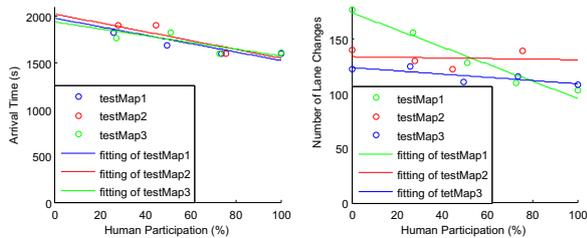
Fig. 10. Preliminary test result from 15 test runs (Road length is 20 km, average distance between traffic vehicles is 120m, average velocity of traffic vehicles is 8.5m/s).
