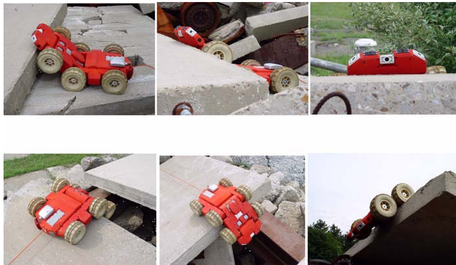
Figure 32 : SPIDAR prototype articulating its chassis/abdomen, sensor head and tilt-camera for (i) better up-above inspection views, and (ii) to perform a crevasse inspection
