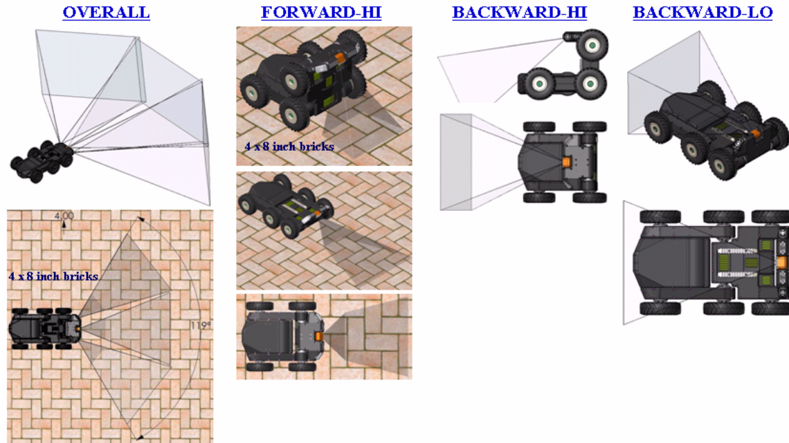
Figure 6 : SPIDAR robot platform FOV configurations for forward camera(s)
