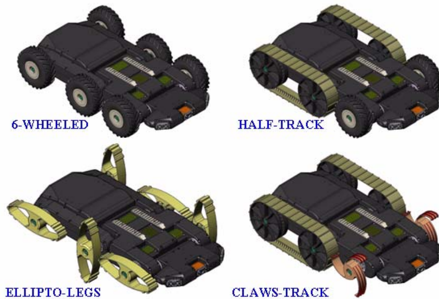
Figure 10 : Possible running-gear configurations for SPIDAR
