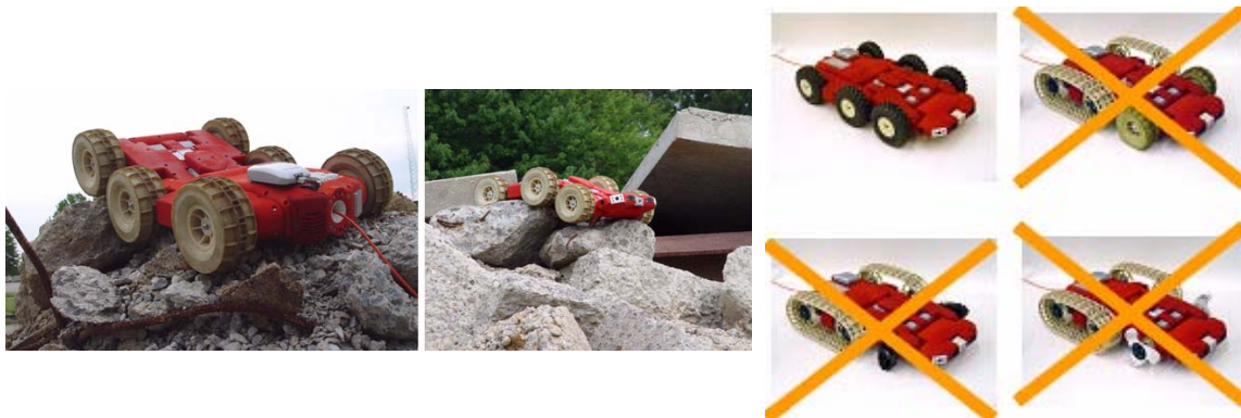
Figure 31 : Multiple locomotor configurations tested; wheeled locomotor deemed most reliable
