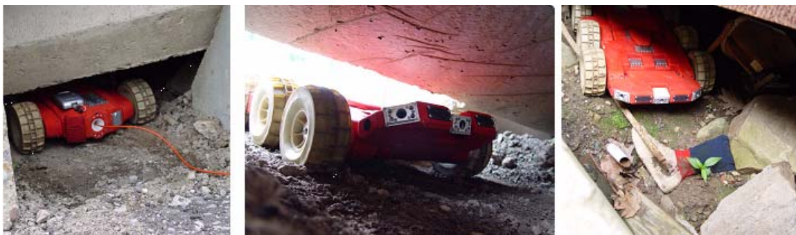
Figure 34 : SPIDAR platform demonstrating extremely constrained space-access, articulation, inspection and search capabilities
