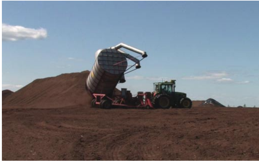
Figure 20. Tractor autonomously dumping at a storage pile that had been acquired using perception.
