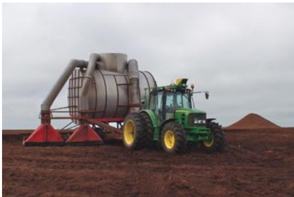
Figure 1. Autonomous tractor with sensor pod and peat moss vacuum harvester, showing a storage pile in the distant background.
