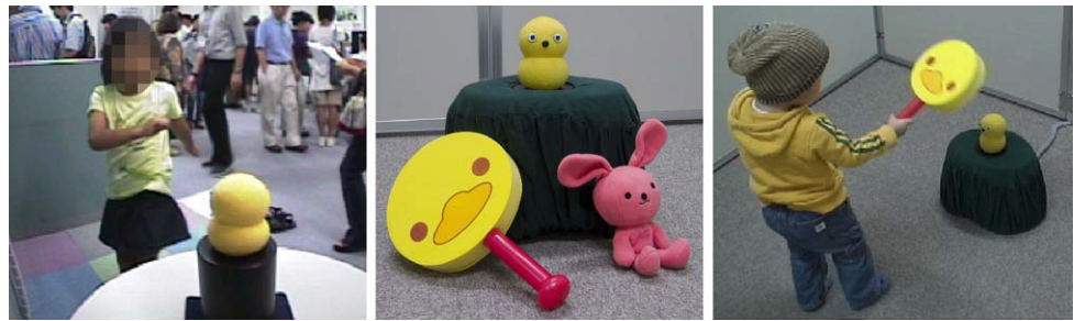
Fig. 13 Keepon dancing with a child using visual movement detection ( left ). Keepon and the two toys used with the accelerometer ( center ): a stuffed rabbit (169 g, 290 mm long) and a soft paddle (137 g, 320 mm long). Keepon dancing with a child holding the paddle ( right )
