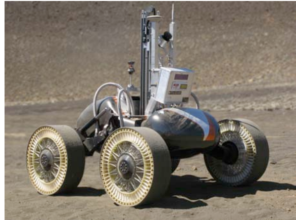
Figure 1. Scarab rover with RESOLVE drill and instrument payload on Mauna Kea, Hawaii
