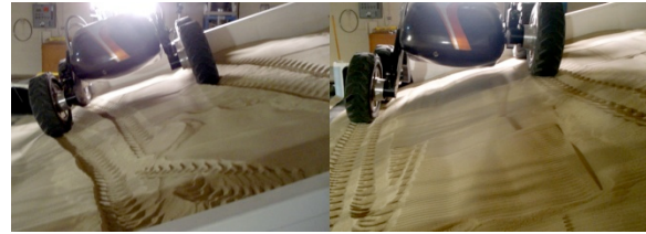
Figure 6. Conventional and Roll Control Cross-Slope Driving showing differences in downhill slip
