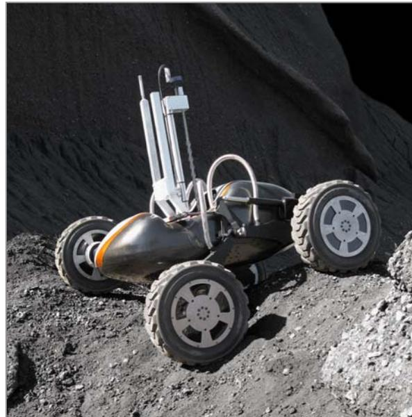
**Figure 7: Suspension conforming to terrain**
