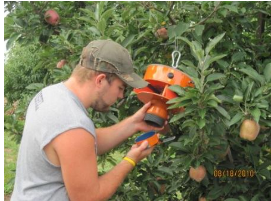
Jason Fissel checks the latest version of the electronic monitoring traps for capturing adult codling moth and oriental fruit moth in apples.
