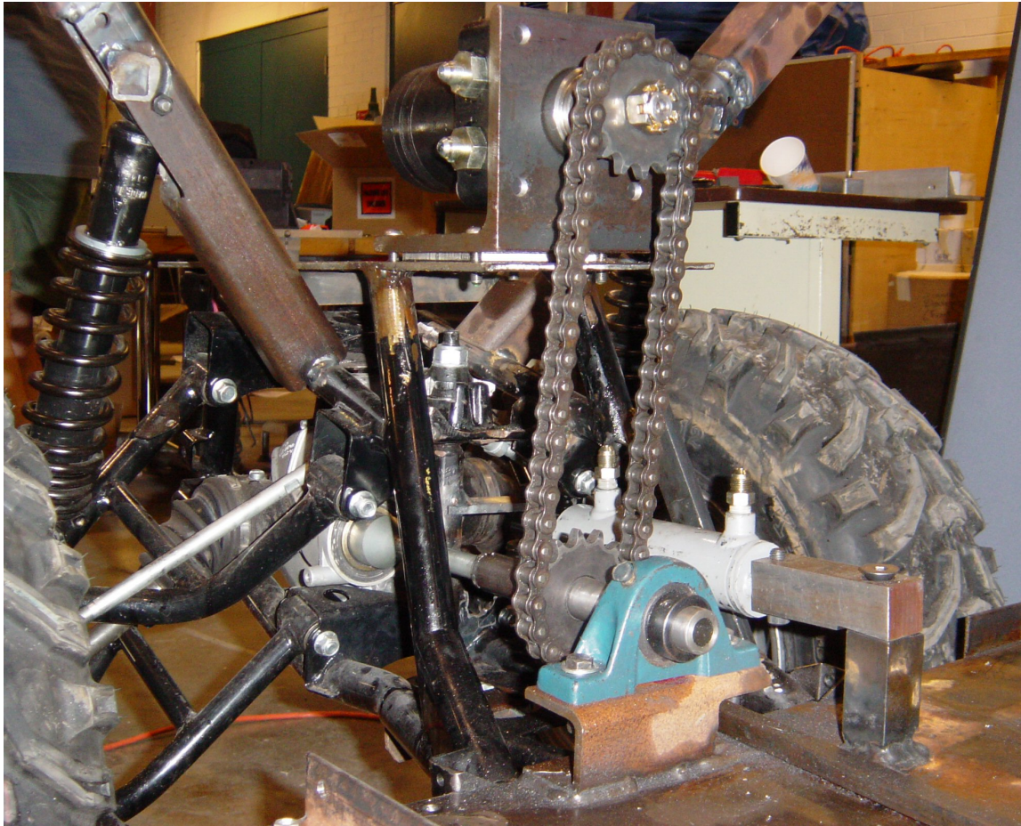
Figure 6.3: Details of Groundhog's steering, drive train and suspension.
