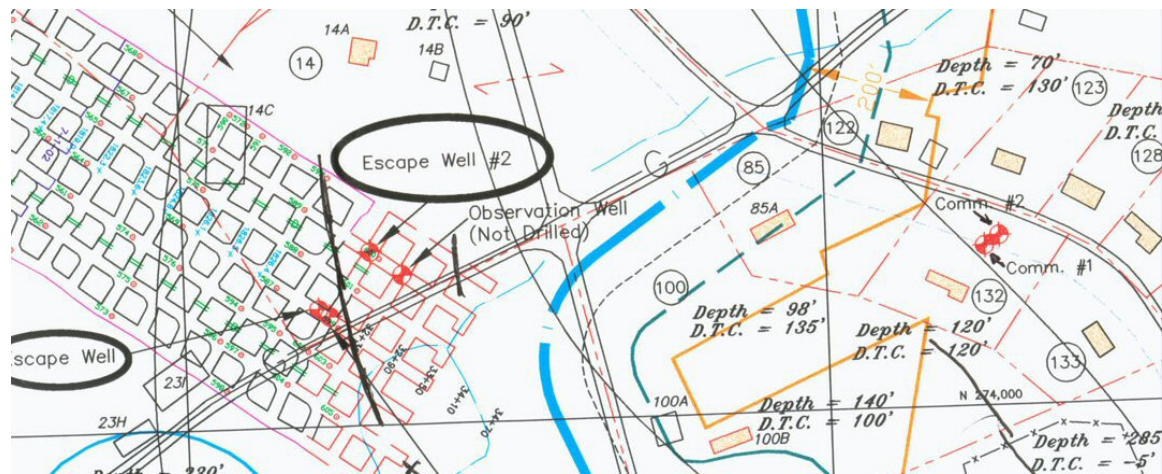
Figure 7.1: Boreholes into the Quecreek and Saxman mines: two 30" diameter rescue holes (left) and two 6" diameter communication holes (right).
