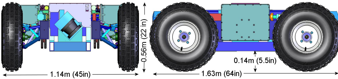
Figure 6.25: CaveCrawler’s low profile enables operations in thin seam mines.
