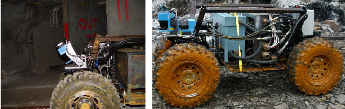
Figure 6.6: Two scanner configurations used for modeling: One of a symmetric pair of nodding line scanners (left), two non-symmetric fixed line scanners (right).
