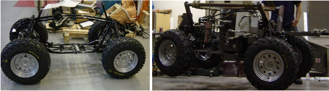
Figure 6.2: Groundhog's base frame with only original ATV components (left) and after additional structural enhancements (right).
