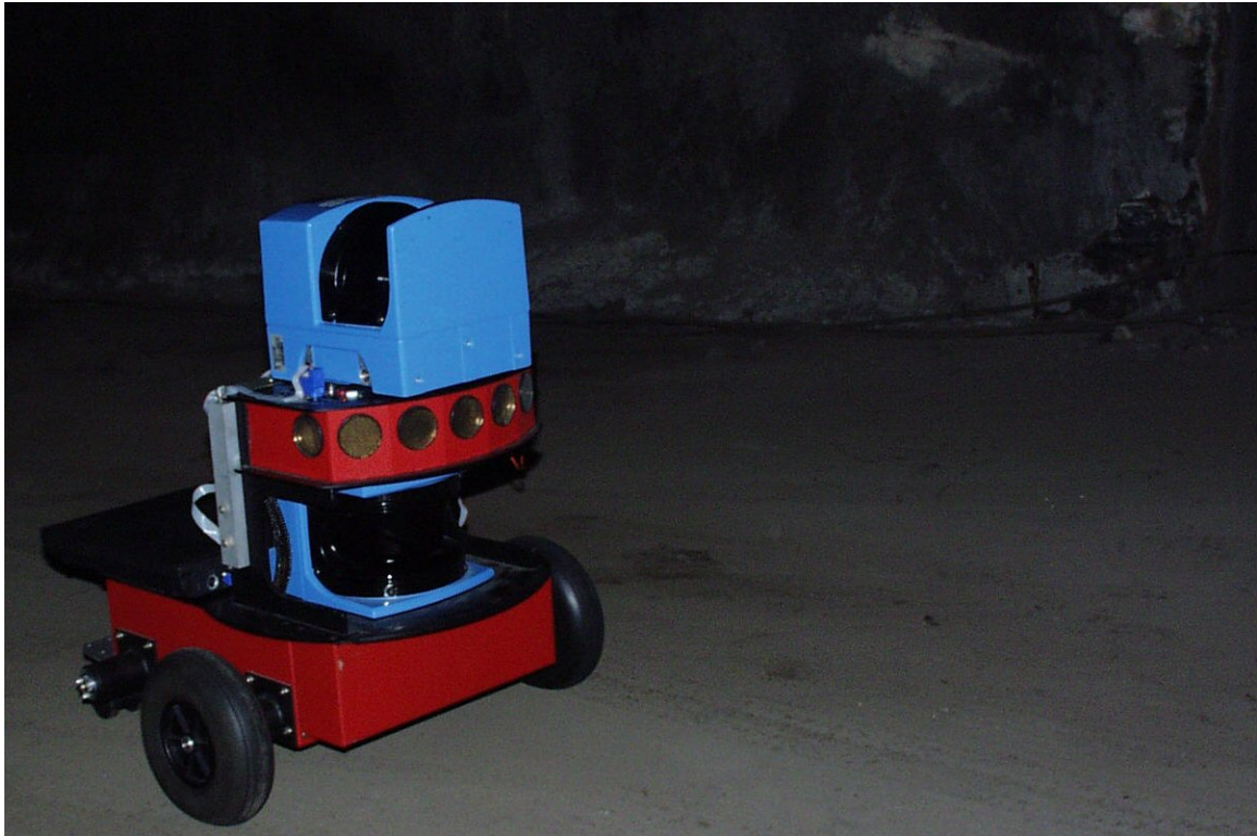
Figure 5.2: A Pioneer-based mobile robot acquiring laser data in a coal mine.
