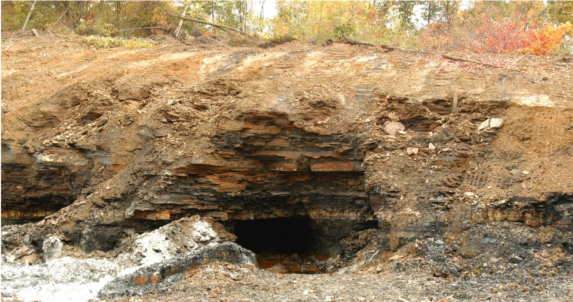
Figure 6.10: Florence Mine, showing exposed abandoned mine corridors protruding from the surface mining high wall.
