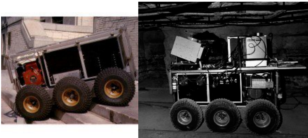
Figure 5.1: The Terregator mobile robots climbing steps(left) and gathering data in a coal mine (right).
