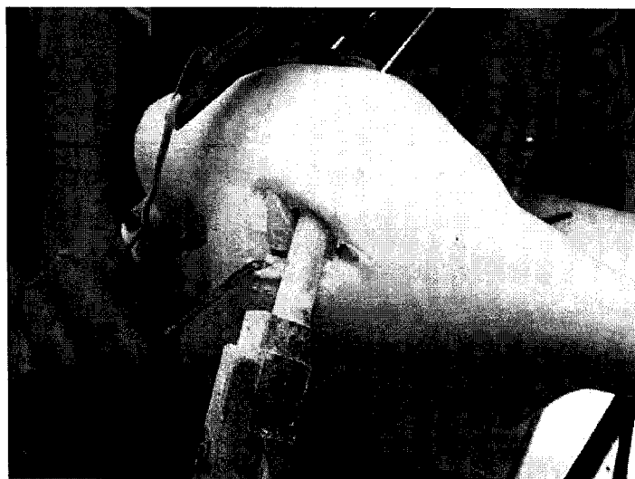
Figure 4-1. PFS operating on sawbones knee covered with foam sheet.
