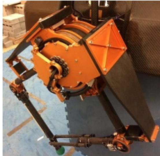
(b) photo of 5-bar mechanism and leaf springs in leg.
