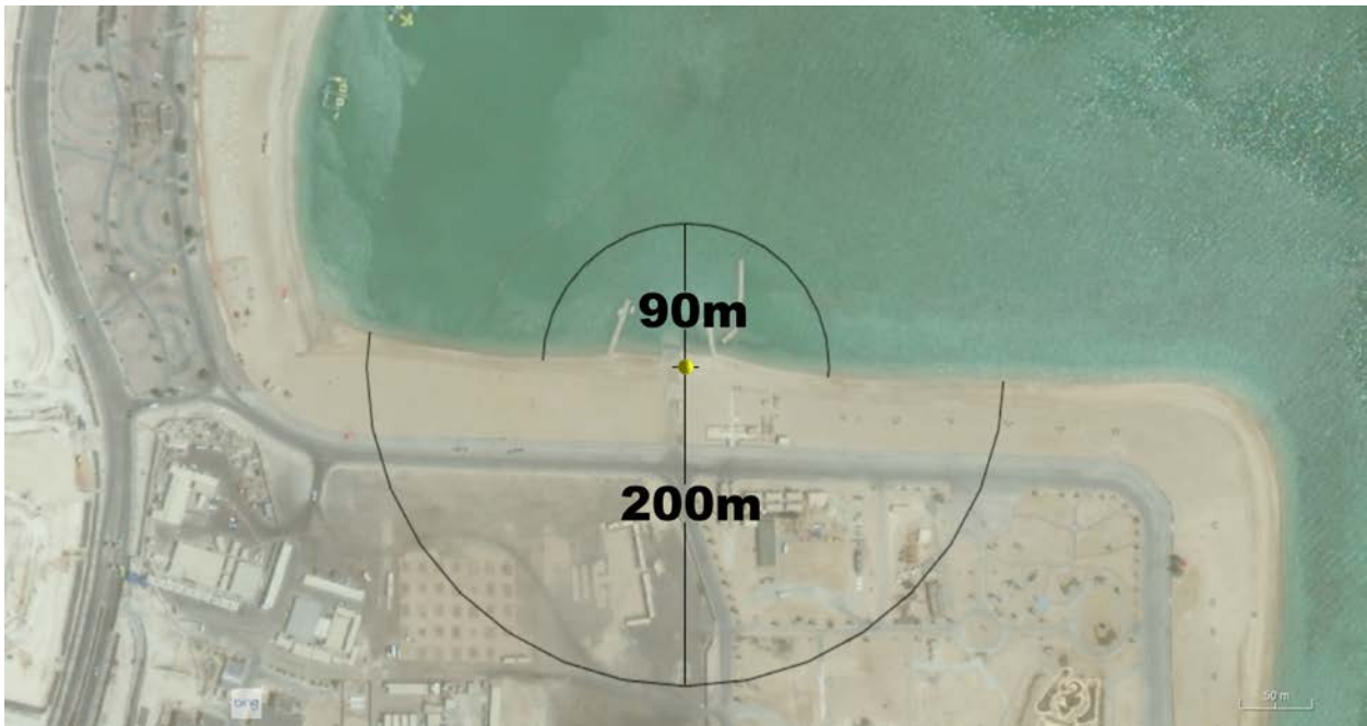
Figure 6.20: Distance (in meters) at which boats can maintain a stable connection to the base station antenna (yellow marker) while floating in the water (top semicircle) versus sitting on the shore (bottom semicircle)
