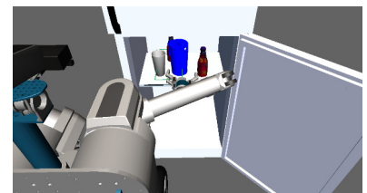
Figure 3.10: An example clearance task. HERB must move the 3 objects in the green rectangle outside the rectangle in order to make space for placing a new item into the refrigerator.
