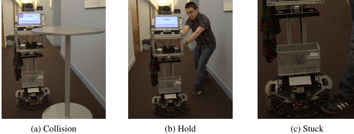
Figure C.1: Types of Motion Interference considered in this work: (a) Collision against a partially detectable obstacle, (b) Being held by a person, and (c) Having one or more wheels stuck
