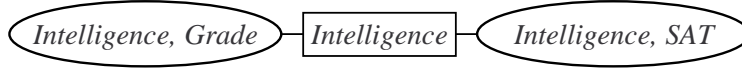
Figure 2.10: A junction tree for the distribution in Figure 2.3(a). The rectangle indicates the separator.
