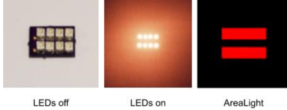
Figure 3.4: Light model comparison: The mesh model of the AreaLight model was chosen to match the real LEDs array set as shown on the left. Our simulation model matches closely in terms of spatially varying illumination obtained on the sensor surface.
