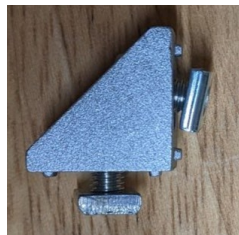
(c) A corner assembly which consists of an off-the-shelf corner bracket, machine screws, and t-nuts pre-assembled to make attachment easier.
