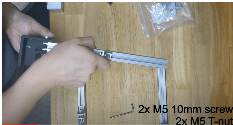
Figure B.1: A screenshot from the RoboLoom assembly instructions showing a step of assembly. The written text document for assembly lists this instruction as “Put the holders onto the bottom square pieces... Put a screw through the holes and each side of the foot holder and screw on a t-nut to each screw. Slide the 8020 into the holder.”
