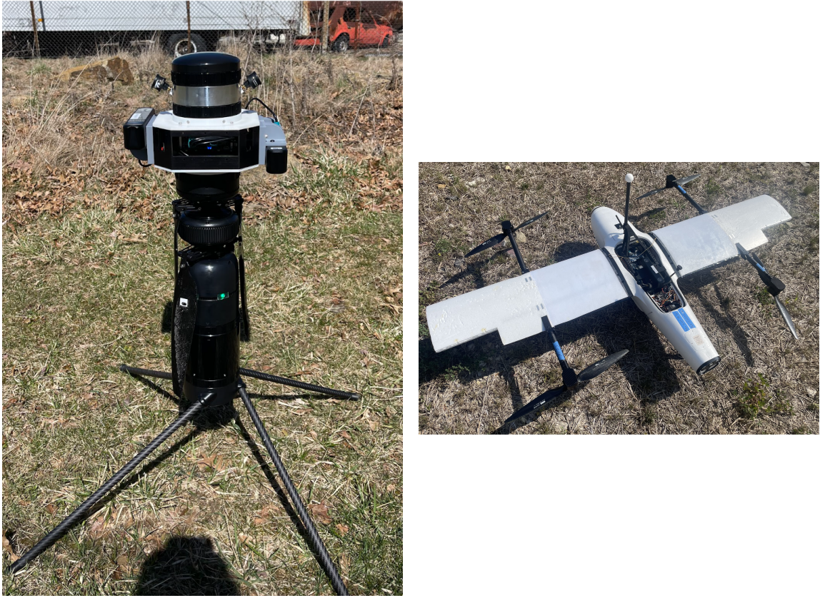
Figure 4.6: Left: A coaxial drone wire data collection platform, Right: a VTOL wire data collection platform
