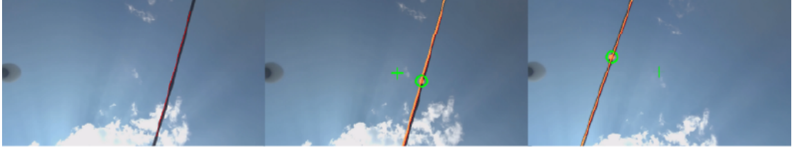
Figure 5.6: Frames from a video sequence demonstrating our wire tracking method on a single-wire scenario. The leftmost image shows the wire beginning to be detected but not yet tracked, while the final two images show the track initialized and maintained across frames
