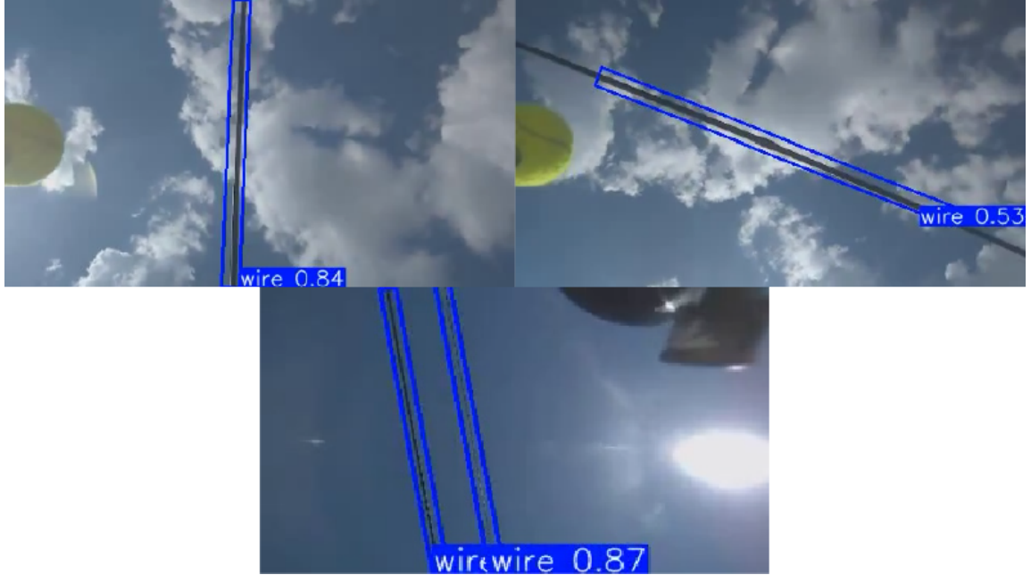
Figure 5.5: Inference examples generated by the fine-tuned YOLO11 oriented bounding box model
