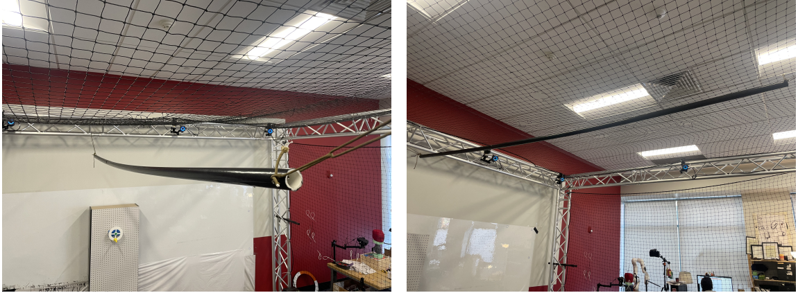
Figure 4.4: Indoor pseudo wire testing setup for controlled single wire testing
