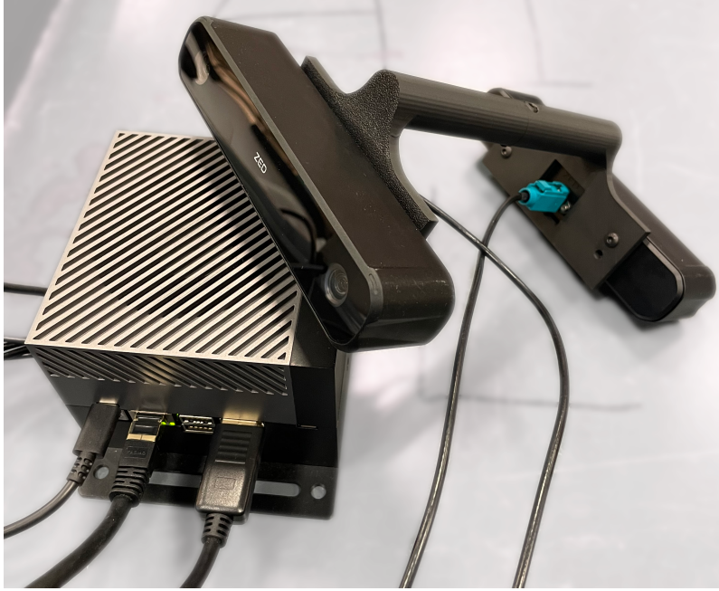
Figure 4.5: Handheld testing jig for wire tracking validation
