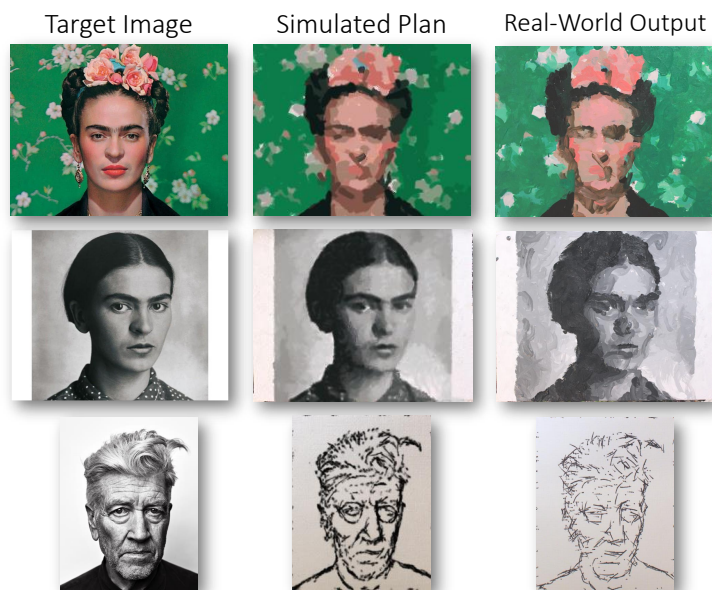
Figure 4.1: FRIDA’s Low-Level Planner is capable of planning of reproducing images. FRIDA is able to plan in simulation to reproduce an image even if it is not possible to be pixel-perfect due to limitations in the robot’s tools. The Sim2Real gap is decreased by using real robot data to inform the simulator. Target image sources: [51, 52, 53].
