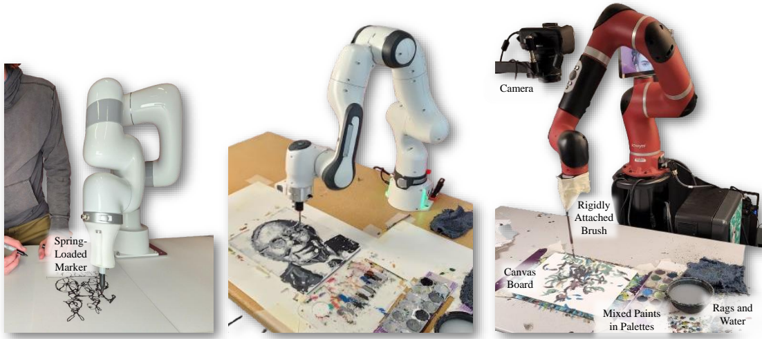
Figure 4.2: FRIDA’s embodiments and workspaces - (Left) Ufactory Xarm Lite6 with a spring-loaded marker holder. (Center) Franka Emika FR3 with a small brush. (Right) Rethink Sawyer with a large brush.
