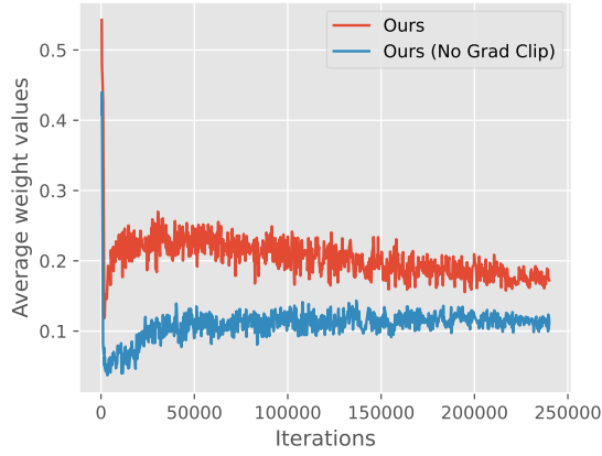
Figure 4.10: We plot the mean weight values of our method and our method without the weight gradient clipping throughout training. We observe a clear reduction in the weight magnitudes in the variant without gradient clipping suggesting a clear positive bias in the weight gradients in this variant. These ablations are performed on the non-streaming 8-step version of the problem.
