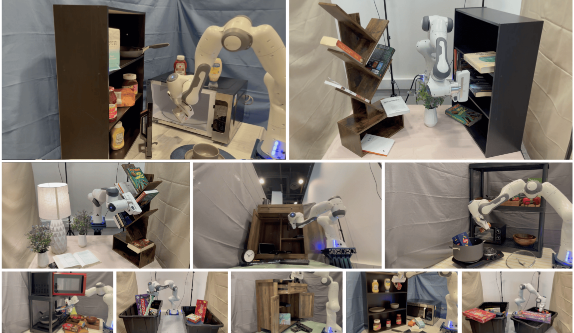
Figure 3.1: Neural Motion Planning at Scale in the Real World Our approach enables a single neural network policy to solve motion planning problems across diverse setups; Neural MP can generate collision free motions for a wide array of unseen tasks significantly faster and with higher success rates than traditional as well as learning-based motion planning approaches.
