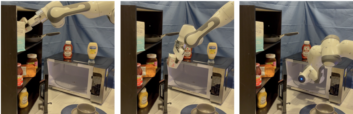
Figure 3.4: Sampling-based planners struggle with tight spaces, a regime in which Neural MP performs well.
