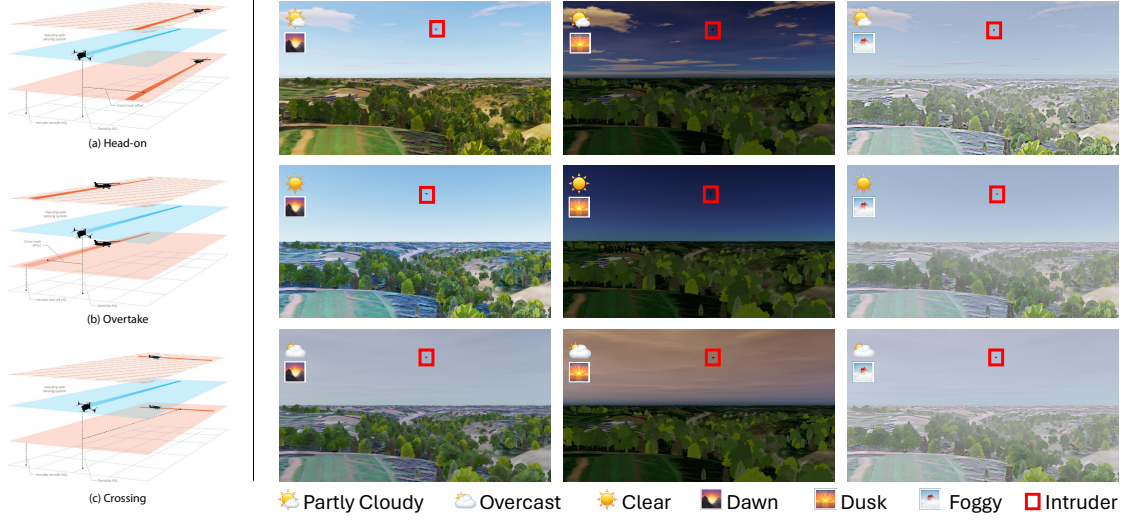
Figure 2.4: Diversity of the airborne collision testing scenarios: (a) The various encounter geometries used for real-world & simulation flight testing. (b) The diverse weather and lighting conditions that were used to evaluate ViSafe 's robustness in simulation. In the simulation, based on the chosen encounter geometry, the intruder position is sampled randomly on the flying corridor.
