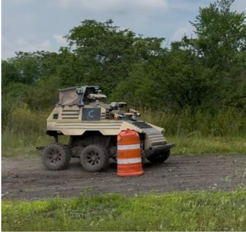
Figure 7.1: Sabrecat navigating around an orange barrel from the left.
