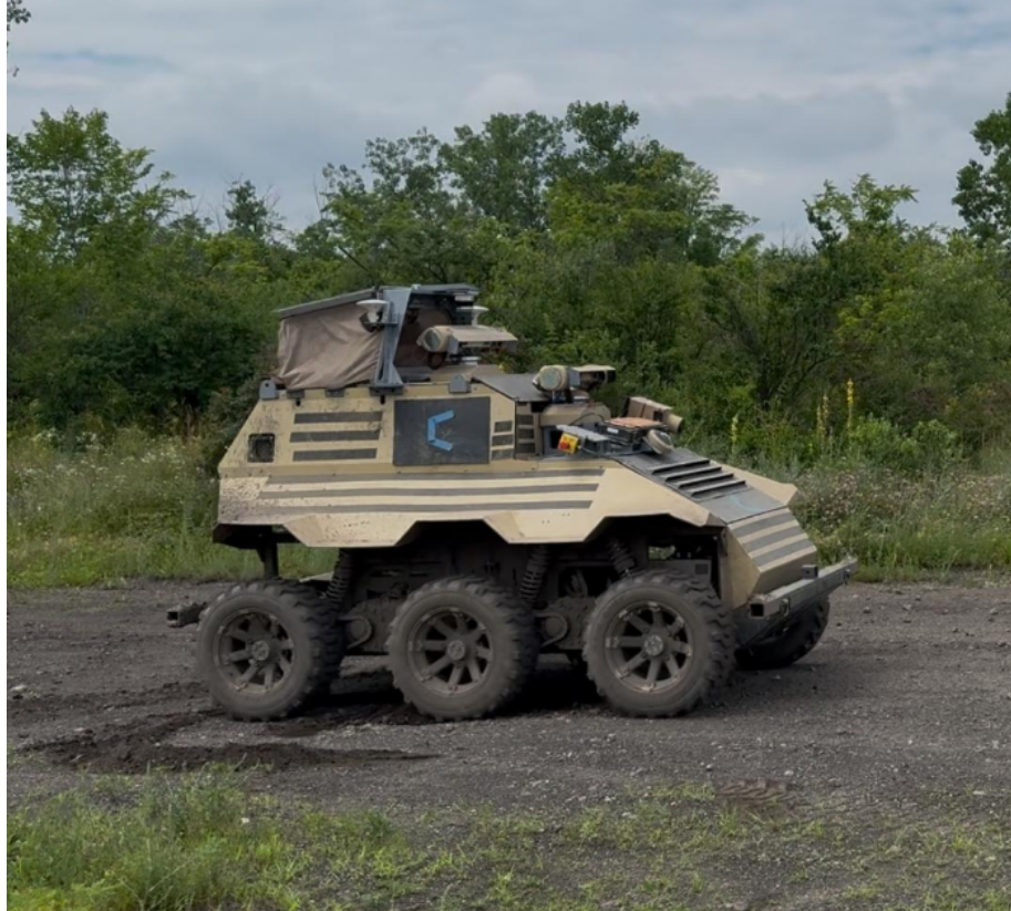
Figure 1.1: Real-world deployment platform used for reinforcement learning experiments. The off-road autonomous vehicle, equipped with onboard sensors and compute, is capable of traversing complex terrains such as gravel, vegetation, and slopes—providing a challenging and realistic testbed for learning-based control algorithms.
