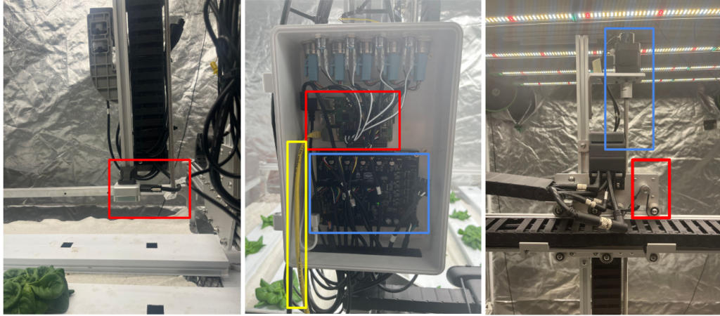
Figure 3.7: The left image shows the end effector of the FarmBot. The middle shows the FarmBot computer (red), an Ethernet connection (yellow), and the motor controller board (blue). The right image shows the belt-driven Y-actuation system (red) and the lead-screw Z-actuation system (blue).
