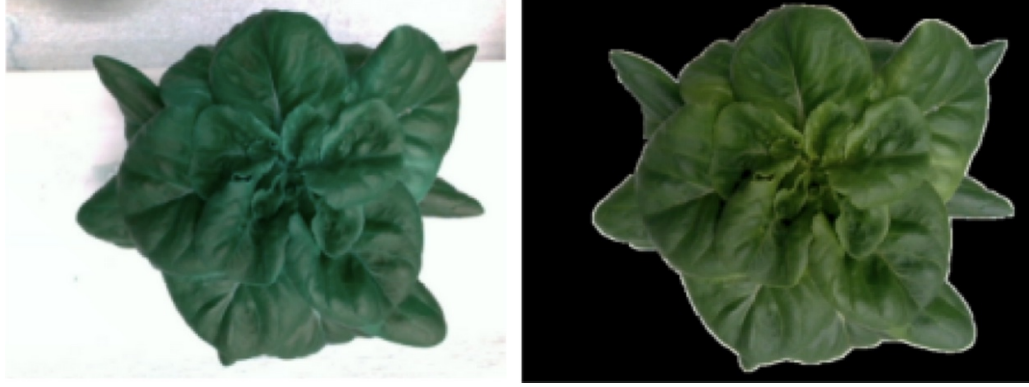
Figure 4.4: Example of converting a sample image on the left into a color-segmented image on the right.
