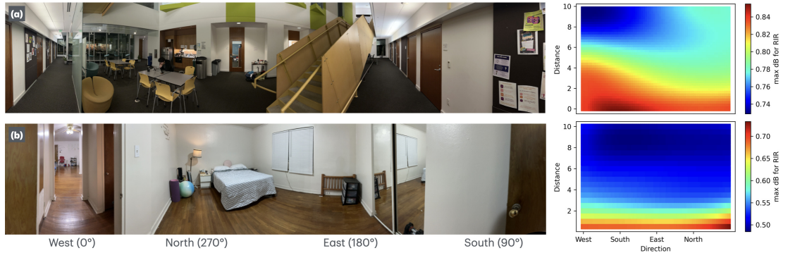
FIGURE 5.7: We present our ANP model’s predictions for maximum decibels of room impulse response (max dB RIR) with real-world panorama scans. Note that max dB RIR is normalized between 0 to 1. Top: a large space in an office building. Here the north faces an open space area, with a corridor from west-to-east direction. There is a staircase close enough in the northeast direction that blocks most of the sound. In the south direction is a wall, and office rooms have closed wooden doors and bulletin boards. Bottom: a bedroom of an apartment. The west direction leads to a corridor and then the living area till 9.5m from the robot’s location. The bed and a side table are placed in the north, with a wall at about 3.5m. Towards the north are windows and some furniture at about 3 m relative to the robot. In the south direction, a wall and an opened wooden door at 0.5m. The sound measurements are reported in Table 5.1. Our model’s predictions align with that sound decays slowly in the open space with distance and peaks at shorter distances in corridors due to reverberations. The decay is much faster in a smaller room than in an open office space.
