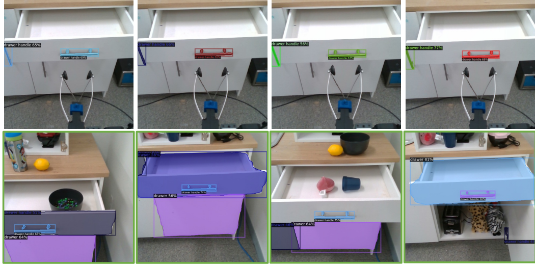
FIGURE C.8: Close drawer task: Showing variability and out-of-domain distribution covered by test against training samples. Top row: Training scenes. Note the absence of any clutter and narrow range of relative positioning of drawer with respect to the camera and robot. Bottom row: Test scenes. Note presence of objects used in other tests in the same frame. Green boundary signifies successful episode, red a failed episode.
