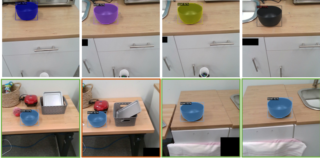
FIGURE C.7: Pour into bowl task: Showing variability and out-of-domain distribution covered by test against training samples. Top row: Training scenes. Note that the bowl was always placed somewhere on this particular region (right of sink) on the counter. Bottom row: Test scenes. Note bowl is surrounded by unseen clutter, placed in novel unseen environment and at relatively different positioning with respect to the camera and robot. Green boundary signifies successful episode, red a failed episode.
