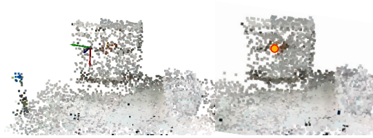
FIGURE 4.6: Output for interaction action predicted by PerAct (left) and interaction point predicted by SLAP (right) for the same input. We see a trend where \pi_I predictions for finer details are consistently more optimal
