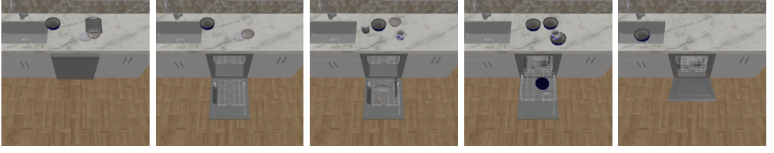
FIGURE 2.4: Dishwasher Loading demonstration in AI Habitat Kitchen Arrange Simulator. Objects dynamically appear on the countertop (ii-iv), and need to be placed in the dishwasher. If the dishwasher racks are full, they land in sink (v).
