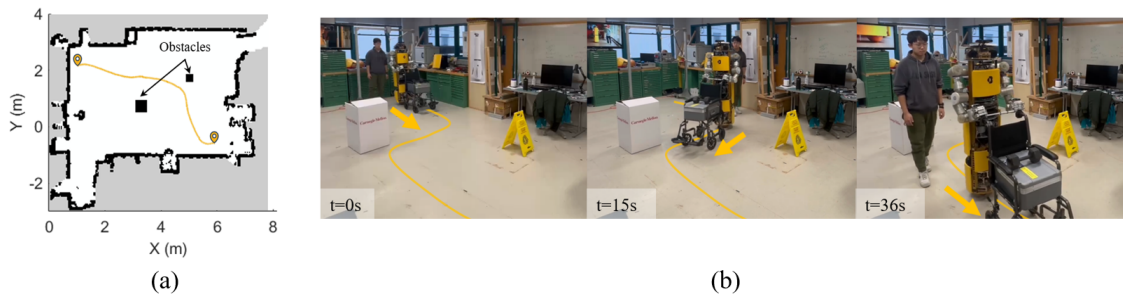
Figure 2.10: Navigation across lab with predefined obstacles. (a) Map with predefined obstacles. The markers indicate the start position (left marker) and goal position (right marker), and the yellow line shows the actual trajectory of the ballbot. (b) Time-lapse picture of the experiment. Yellow arrow indicates ballbot’s velocity direction.
