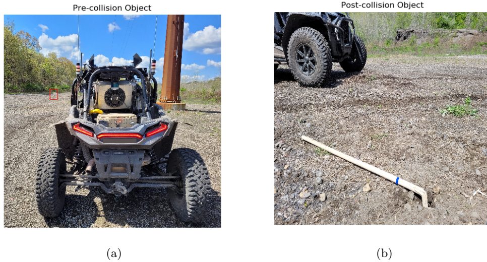
Figure 6.7: Two images of the 25.4 [mm] post used in the second experiment. Figure 6.7a demonstrates the condition of the object before being struck by the vehicle. Figure 6.7b demonstrates the condition of the failed object after being struck by the vehicle.
