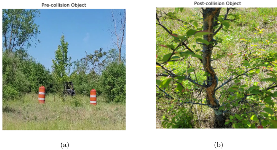
Figure 6.9: Two images of the 81.8 [mm] tree overridden in the third experiment. Figure 6.9b demonstrates the condition of the object before being struck by the vehicle. Figure 6.9b demonstrates the condition of the failed object after being struck by the vehicle.
