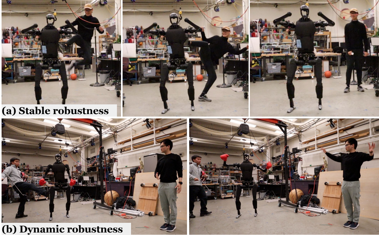
Figure 8.7. Robustness Tests of our H2O system under powerful kicking. The policy is able to maintain balance for both stable and dynamic teleoperated motions.
