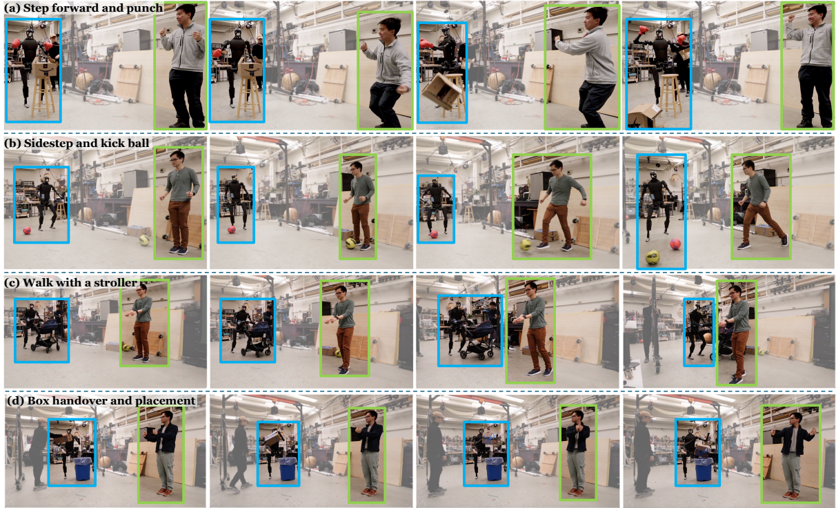
Figure 8.4. The humanoid robot is teleoperated in real-time using an RGB camera by the human teleoperator . (a) The humanoid mimics the human teleoperator, advancing one step while delivering a punch to displace a box, followed by a victory gesture. (b) The humanoid executes a precise sidestep to align with a ball and delivers a controlled kick using its right foot. (c) The humanoid demonstrates forward walking while pushing a stroller. (d) The operator teleoperates the humanoid to catch a box, rotate its waist, and drop the box into a waste bin. Videos: see the website .
