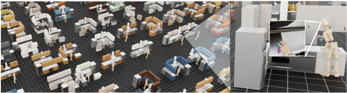
Figure 7.1. Perceptive Dexterous Control (PDC) enables a humanoid equipped with egocentric vision to search for, reach, grasp, and manipulate objects in cluttered kitchen scenes. We use visual perception as the sole interface for indicating which hand to use, which object to grasp, where to move, and which drawer to open.
